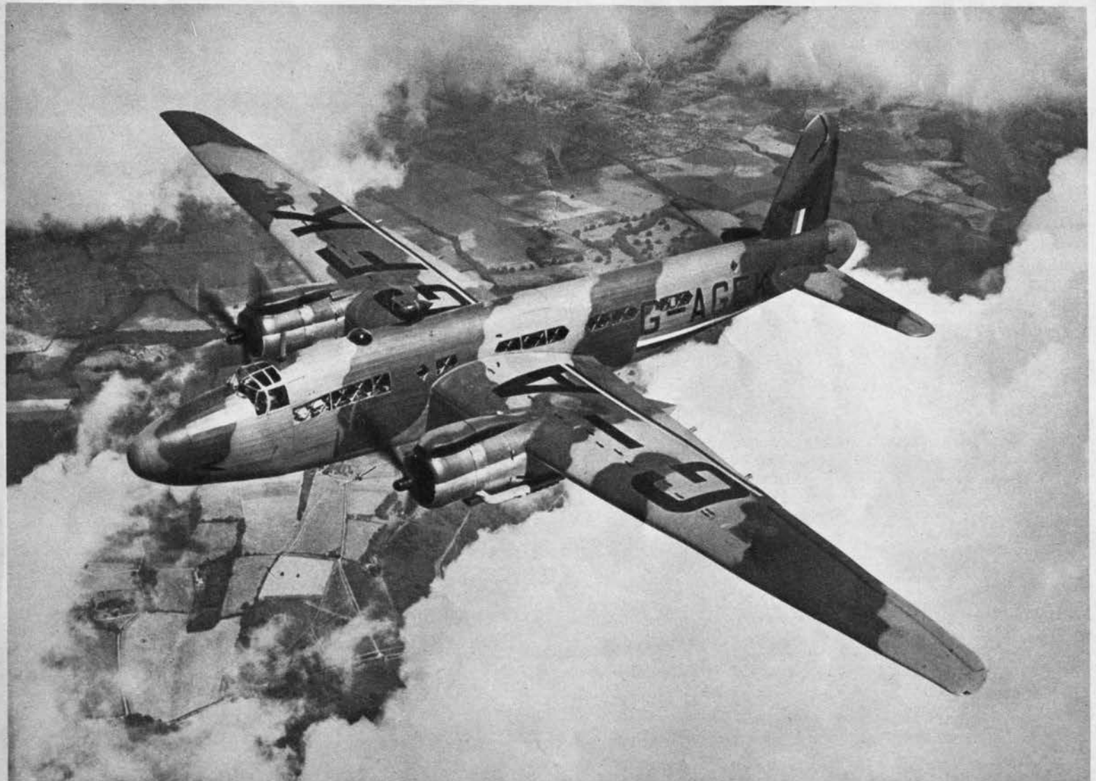
Anglo-American co-operation made the Warwick possible. Its two engines are U. S.-built, the airframe English. Geodetic structure of
